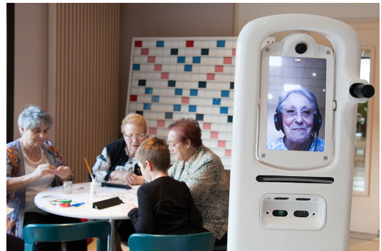
Fig. 1: A telepresence robot for elderly care. The robot in this picture is used to remotely assist with the activities of a day care centre.
